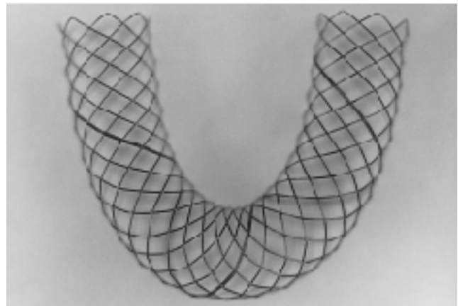
Fig. 5. Flexibility of the new nitinol stent. The lumen did not decrease when the stent was bent to a direction of 180 degrees.
