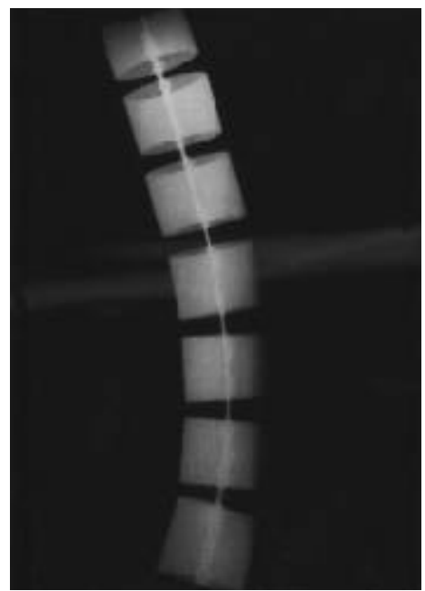
Fig. 2. Conventional lateral radiograph of spine phantom. This phantom was taken at the height of 15cm between table and mid-level of phantom, and at 200mA, 95kVp, 0.3sec with a tube-film distance of 105cm, centered on fifth level of phantom.
