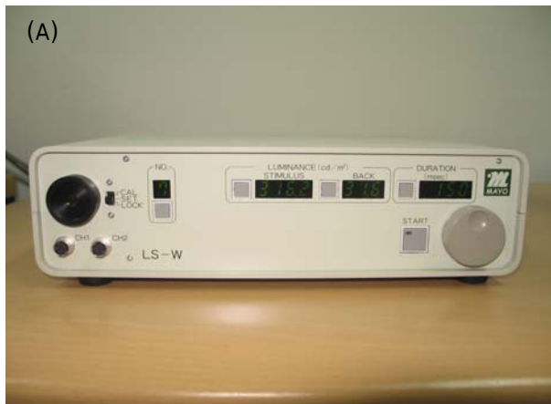
Figure 1. (A) LED-driver (size 20W×16D×6H cm, weight 800 gm; Mayo Co., Nagoya, Japan), (B) contact lens electrode with build-in white LEDs.
