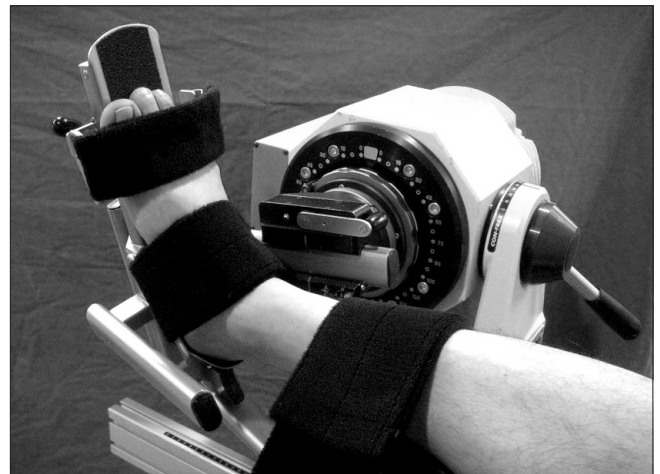
Figure 2. Con-Trex dynamometer (CMV AG, Dubendorf, Switzerland) was used to measure isometric and isokinetic ankle strengths.
