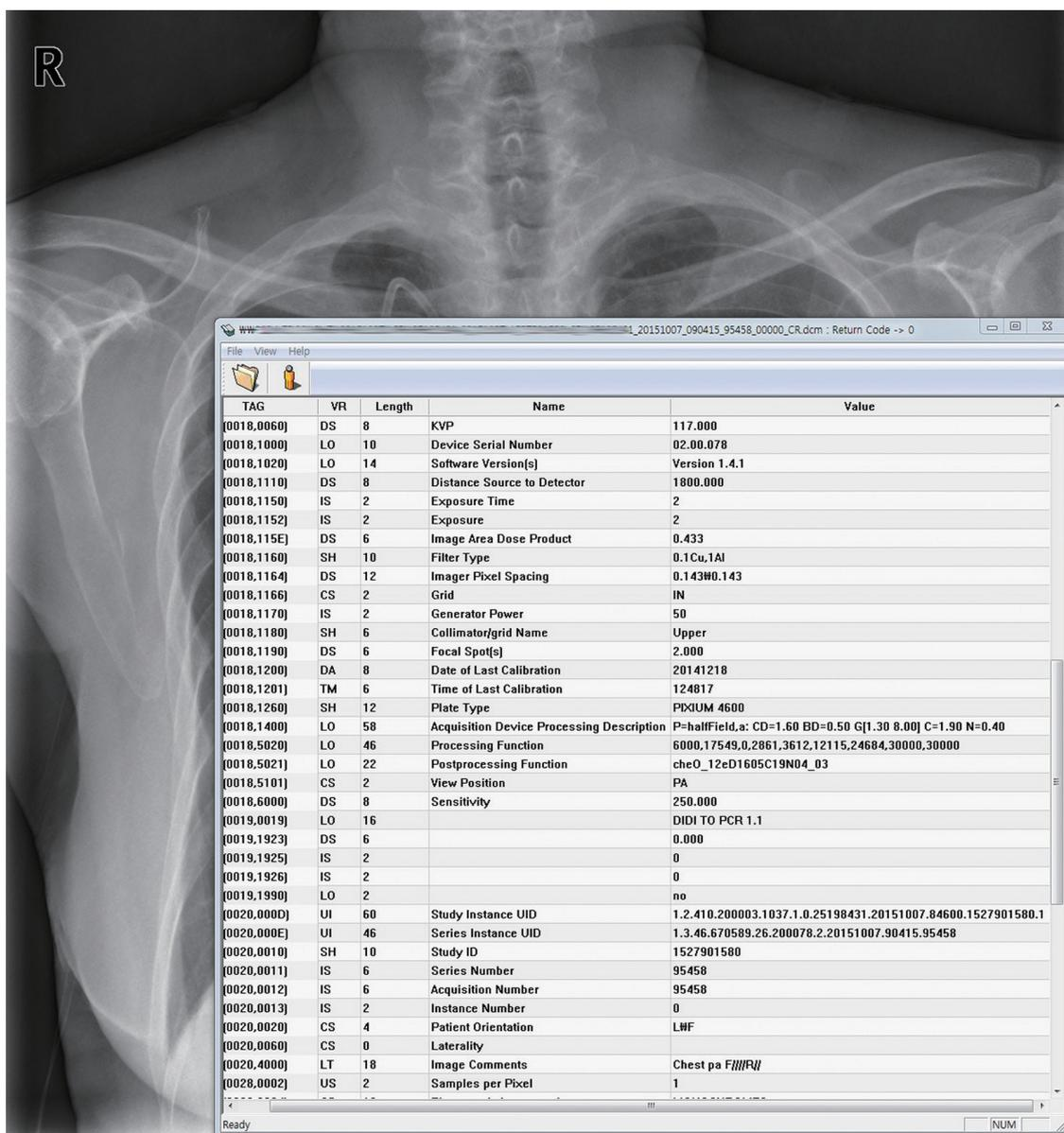
**Fig. 1.** An example of DICOM header of a chest X-ray that includes kVp, mAsm and DAP. The DICOM header shows a kVp value of 117 and DAP of 0.433.
