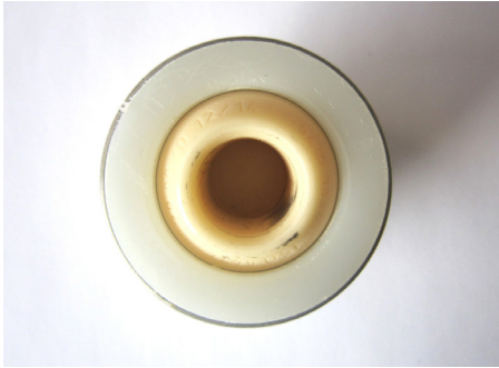
Figure 6. Ceramic on polyethylene articulation.
