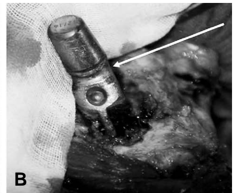
Fig. 5. (A) A rim fracture and metal staining of the ceramic liner and multiple fragments of the ceramic head and (B) a deep groove (white arrow) was observed on the lateral base of the femoral stem.
