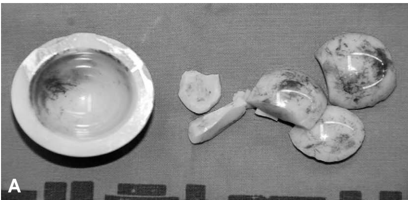
Fig. 5. (A) A rim fracture and metal staining of the ceramic liner and multiple fragments of the ceramic head and (B) a deep groove (white arrow) was observed on the lateral base of the femoral stem.
