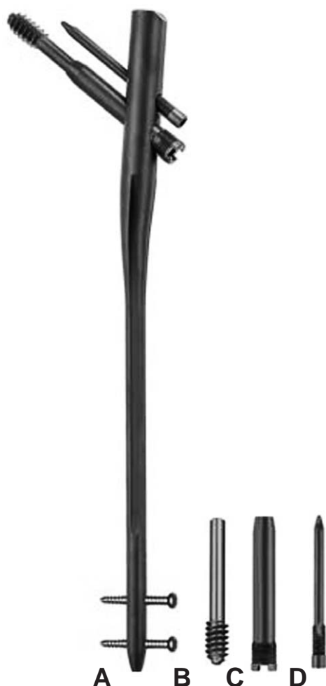
Fig. 1. (A) Targon® proximal femoral nail (PFN, Aesculap, Germany) (B) Lag screw (C) Sleeve (D) Antirotation hip pin.
