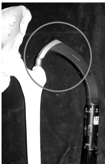
Fig. 5. Gamma 3 nail, curved flexible target device allow small incisions, preventing soft tissue pressure and collision with iliac crest.
