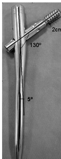
Fig. 1. The ITST (Zimmer) with lag screw. 2 cm of threaded lag screw length, 130° of neck-shaft angle, 5° of medial-lateral angle.
