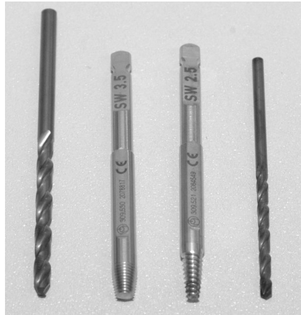
Fig. 2. Conical extraction screws and drills for the removal of the stripped head 16) (Oh et al, with permission).
