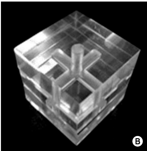
Fig. 1. Schematic diagram of the injectability test (A) and acrylic mold for the rheological test (B).
