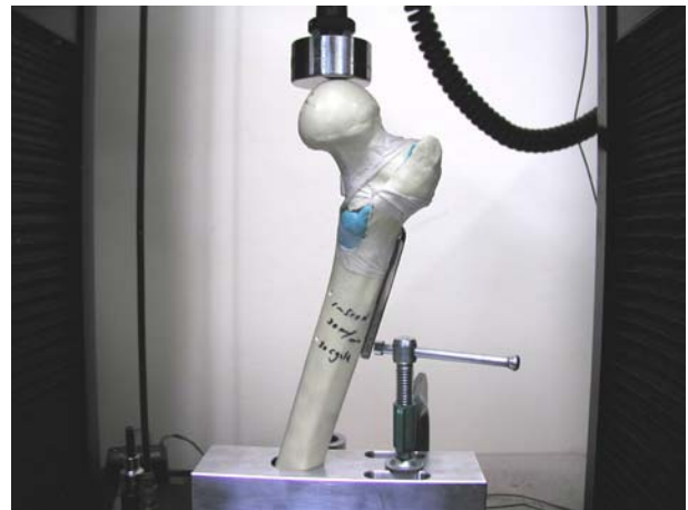
Fig. 4. Bone-plate complex applied on the Instron 6022. (F=500N, Cycle=30 times, Head down velocity=30 mm/min)
