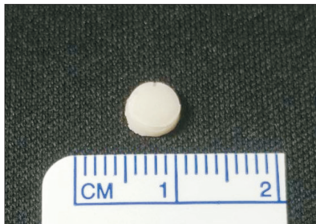
Figure 1. The antibiotics-impregnated cements were manufactured as a disk form 6 mm diameter and 2 mm height.
