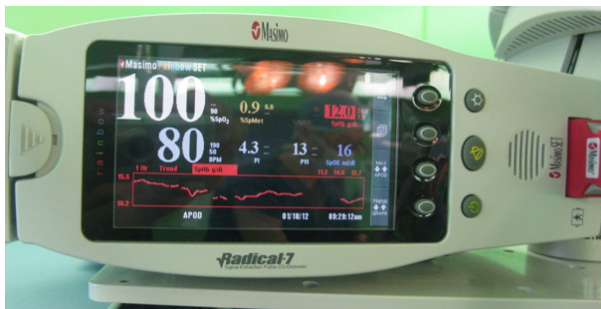
Fig. 1. Masimo Radia-7. It can measure total hemoglobin continuously using pulse oximetry sensor
