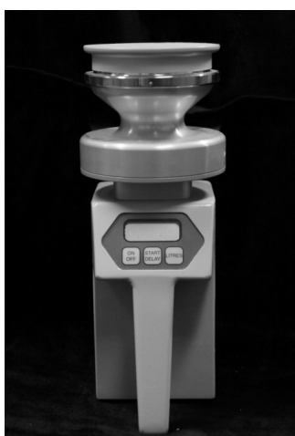
Figure 1. Air sampler (M Air T™, Millipore Corp., Massachusetts, USA) for inhaling the aerosols produced by ultrasonic scaler before, during or after the treatment. The trypticase-soy agar plate is installed at the entrance of the air sampler.
