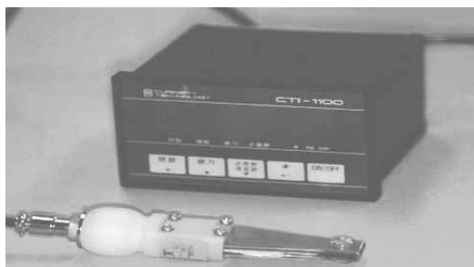
Figure 1. The photograph of Jaw Force Transducer CTI-1100
