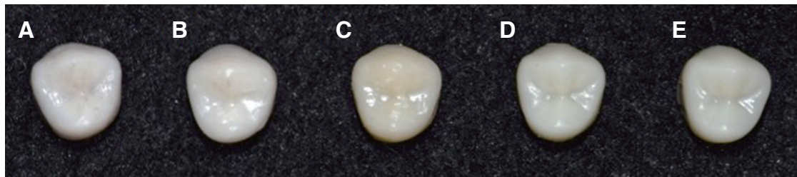
Fig. 1. Specimens prepared by each method for fracture strength test. (A) S3Z, (B) D3Z, (C) D3P, (D) MIL, (E) CON. S3Z, Resin printed by ZENITH SLA 3D printer; D3Z, Resin printed by ZENITH DLP 3D printer; D3P, Resin printed by PROBO DLP 3D printer; MIL, milled resin; CON, conventionally self-cured resin.
