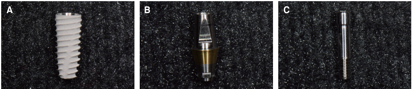
Fig. 1. Materials used in the experiment. (A) Implant, (B) Abutment, (C) Abutment screw.
