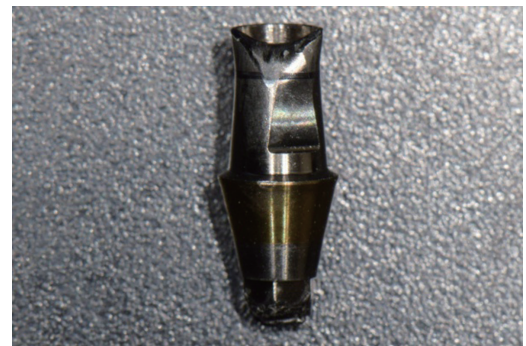
Fig. 7. Fractured abutment screw at the shank area.
