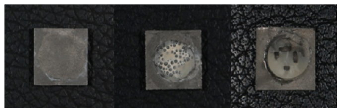
Fig. 6. Ni-Cr alloy specimen surfaces after shear bond strength measurement (In order of flatting, bead and loop).
