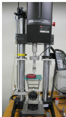
Fig. 2. Push-out test.
