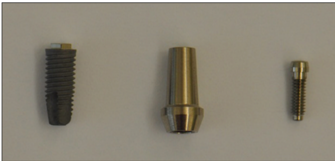
Fig. 4. Implant fixture, abutment, abutment screw used for this study.
