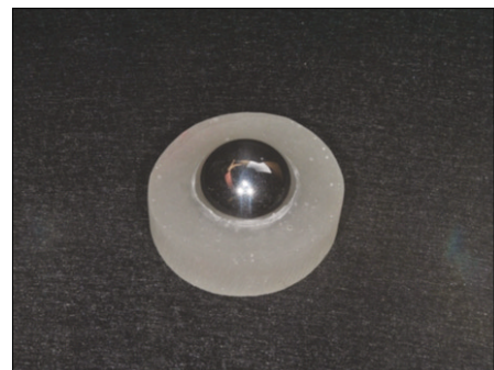
Fig. 2. Ball attachment for flexural load test.
