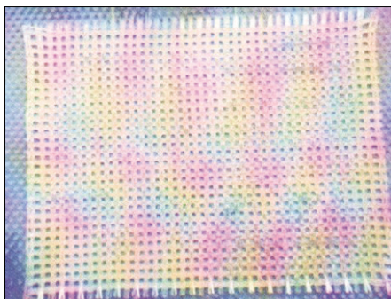
Fig. 1. SES MESH used in this study. 85 - 90% of the mesh is made up of a glass fiber.
