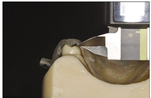
Fig. 7. Measuring the gap between the surgical guide and the model to evaluated the fitness.
