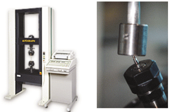
Fig. 3. Universal testing machine for static loading test (AGS-1000D, SHIMADZU Co., Japan).
