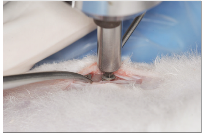
Fig. 3. A photograph of the removal torque test holding the sample. The driver is connected to the implant and the jaws of the digital torque gauge (Mark-10, USA).
