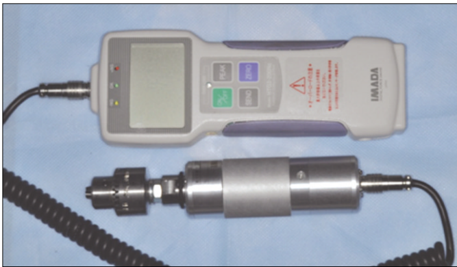
Fig. 2. Digital torque gauge used in this study.
