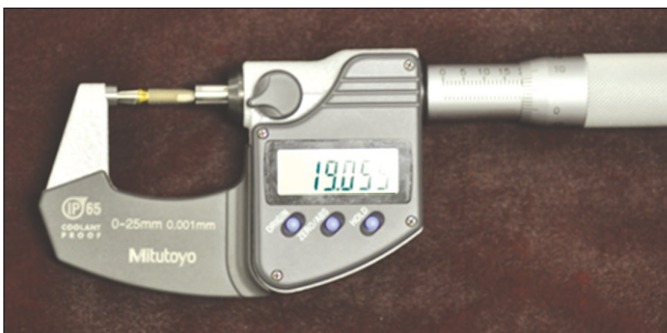
Fig. 3. Measurement of implant-abutment length.
