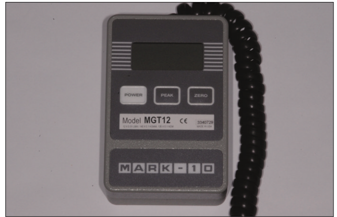
Fig. 4. Digital torque meter (MGT 12; Mark-10 Corp., Copiague, NY, USA).
