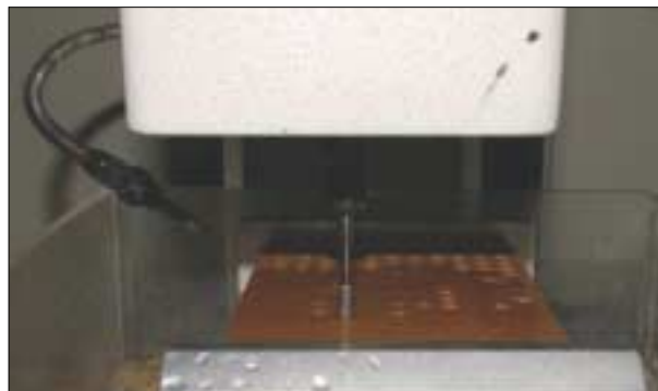
Fig. 2. Forming of insertion hole with auto drilling machine.
