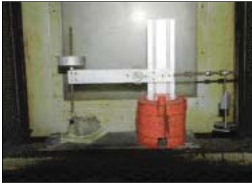
Fig. 5. Loading device located in the stress freezing furnace.
