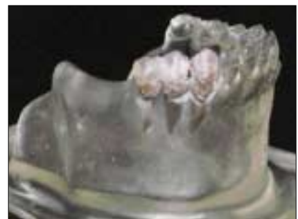
Fig. 3. Photoelastic model with the duplicated resin teeth.
