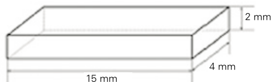
Fig. 1. Dimension of ceramic specimen.
