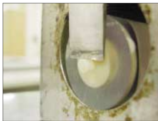
Fig. 2. Specimen in Instron machine (Bonding failure were conformed to measure shear bond strength between resin block and dentin).
