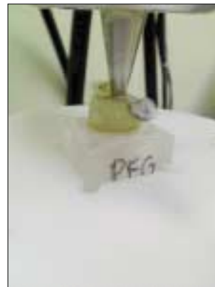
Fig. 6. MTS 858 Bionix II applying cyclic load.
