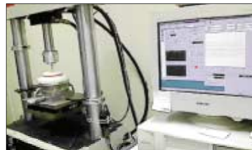
Fig. 6. MTS 858 Bionix II applying cyclic load.
