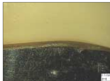
Fig. 5. Measurement of the marginal discrepancy using the video microscope system after internal adjusting and sintering ( \times 100 ).
