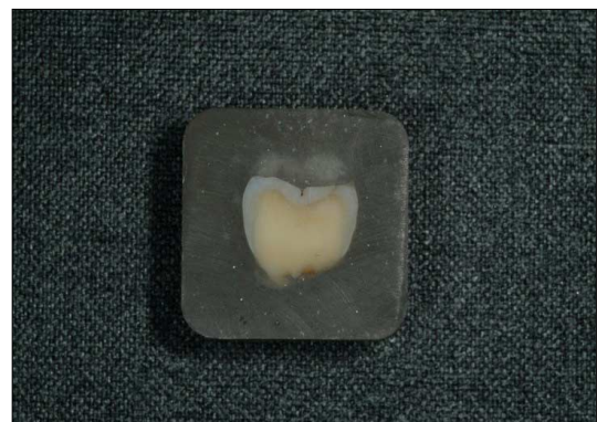
Fig. 1. Impregnated tooth specimen in acrylic resin.
