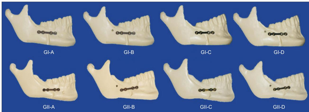
**Fig. 2.** GI, linear osteotomy; GII, angular osteotomy. Subgroups: A, one 4-hole 2.0 mm plate; B, one 4-hole 2.0 mm plate and one bicortical screw; C, one 4-hole 2.0 mm locking plate; D, one 4-hole 2.0 mm locking plate and one bicortical screw.
