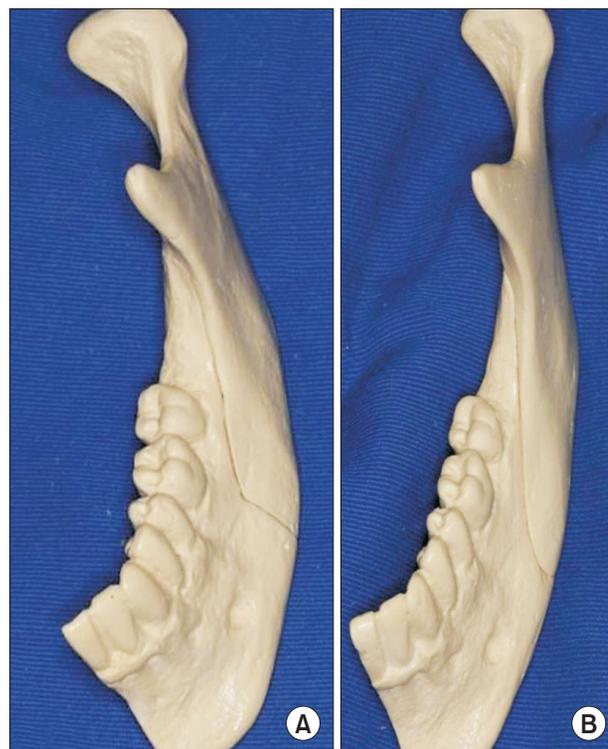
**Fig. 1.** Polyurethane hemimandibles according to sagittal split ramus osteotomy design. A. Group I, right angles between osteotomies. B. Group II, no angles between osteotomies.
