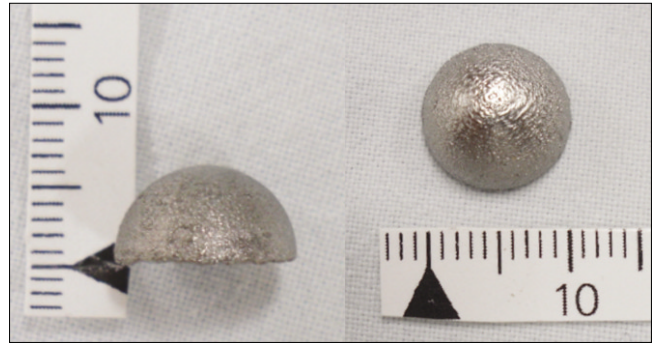
Fig. 1. Rapid prototype titanium cap is 5 mm in height, 10 mm in diameter and 1 mm in thickness with rough surface.
