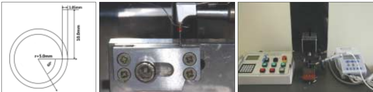
Figure 1. Schematic diagrams and pictures of an artificial canal and a fatigue tester (Denbotix).
