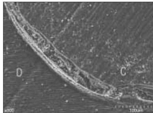
Figure 3-d. SEM image of Filtek flow specimen with a gap in the bonding interface.
