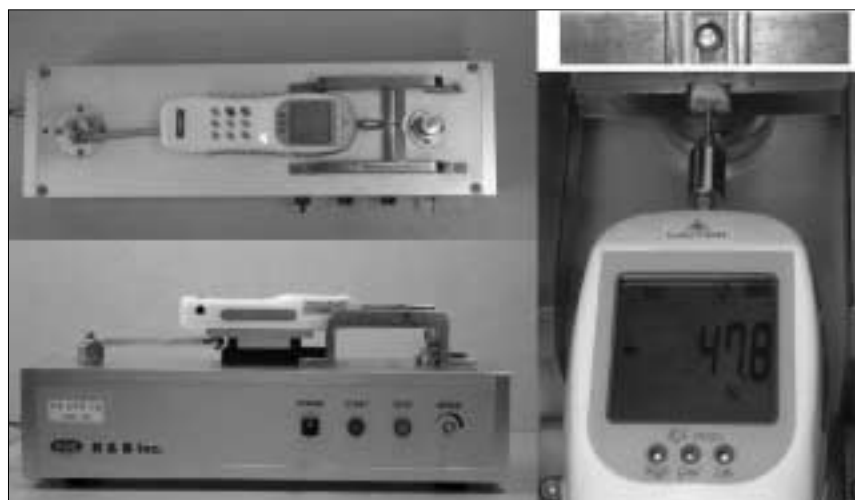
Figure 2. Push-out bond strength measuring device.
