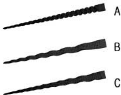
Figure 2. Final FE models of three NiTi files used in this study: A: ProFile .06 / #30, B: ProTaper F3, C: ProTaper Universal F3.
