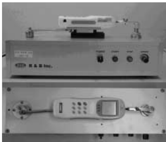
Figure 1. Shear bond test machine.
