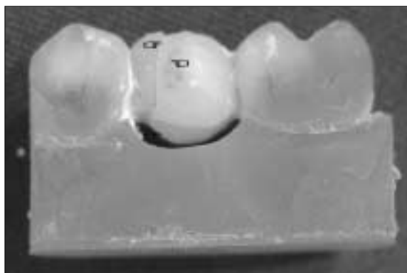
Figure 7a. Vertical fracture on the pontic tooth area.
