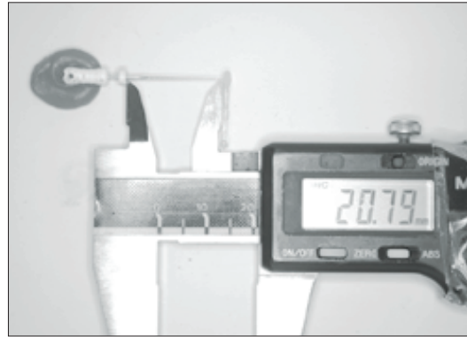
Figure 2. Length measurement with Digital caliper.
