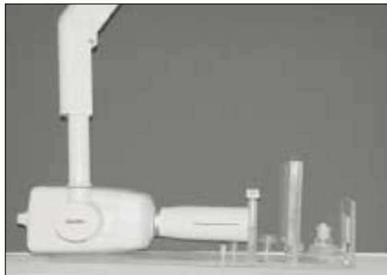
Fig. 5. Geometrically standardized experimental design. A: tube head of Gendex intraoral X-ray unit, B: acrylic resin plate with hole block of tooth, C: 2cm thick acrylic block simulating the soft tissue.
