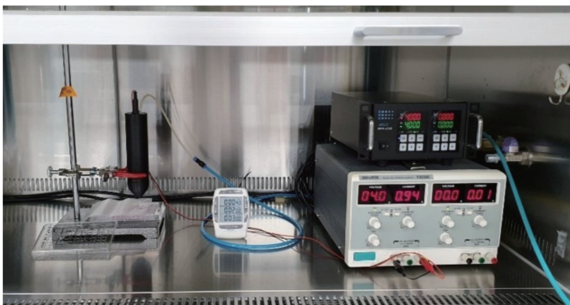
Fig. 1. Customized helium gas non-thermal atmospheric pressure plasma equipment for in vitro study.
