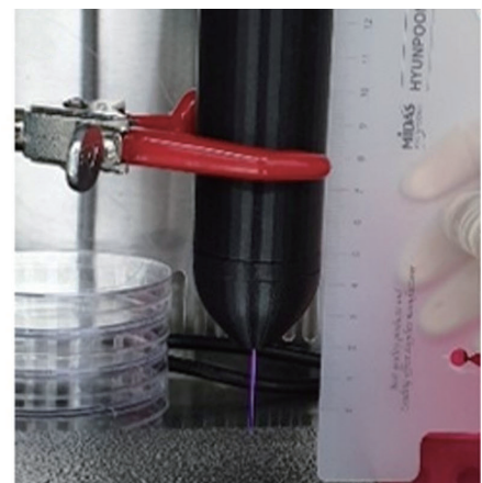
Fig. 1. Customized helium gas non-thermal atmospheric pressure plasma equipment for in vitro study.
