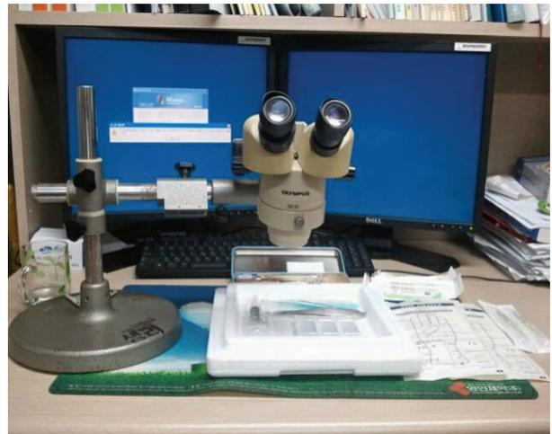
**Fig. 2.** A desktop medical school laboratory microscope with fixed magnification is used for the anastomosis training because it is easily available from the school or the hospital. The magnifications of the microscope are 10× and 30×. The 10× magnification is primarily used.
