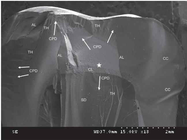
**Fig. 6.** SEM fracture surface image of SU crown with occlusal thickness of 1.5 mm. HL: hackle line, AL: arrest line, CC: compression curl, TH: twist hackle, white star: origin of fracture, white solid arrow: crack propagation direction (CPD), CL: cementation layer, SD: supporting die.
