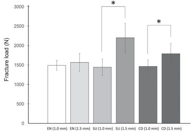
**Fig. 3.** Means and standard deviations of fracture loads of ceramic groups with different occlusal thickness conditions (1.0 mm and 1.5 mm). Significant differences ( $P < .05$ ) between the groups were evaluated with independent t-tests and marked with asterisks. EN - Enamic, polymer-infiltrated-ceramic network, SU - Suprinity, zirconia-reinforced lithium silicate, CD - Celtra Duo, zirconia-reinforced lithium silicate.
