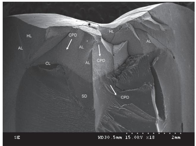
**Fig. 8.** SEM fracture surface image of EM crown with occlusal thickness of 1.5 mm. HL: hackle line, AL: arrest line, CC: compression curl, TH: twist hackle, white star: origin of fracture, white solid arrow: crack propagation direction (CPD), CL: cementation layer, SD: supporting die.
