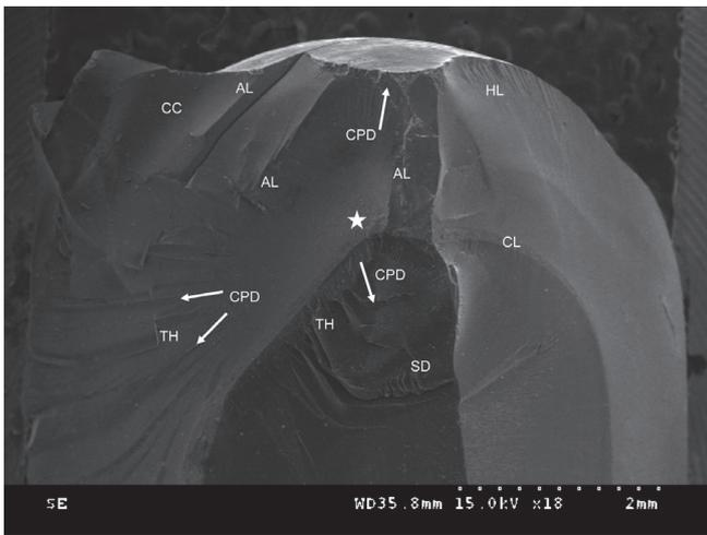
**Fig. 7.** SEM fracture surface image of CD crown with occlusal thickness of 1.5 mm. HL: hackle line, AL: arrest line, CC: compression curl, TH: twist hackle, white star: origin of fracture, white solid arrow: crack propagation direction (CPD), CL: cementation layer, SD: supporting die.
