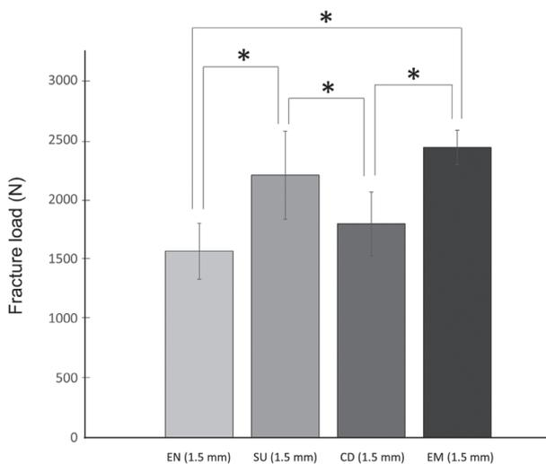
**Fig. 2.** Mean and standard deviations of fracture loads of ceramic groups with the same occlusal thickness (1.5 mm). Significant differences ( $P < .05$ ) between the groups were evaluated with Tukey HSD test and marked with asterisks (\*). EN - Enamic, polymer-infiltrated-ceramic network, SU - Suprinity, zirconia-reinforced lithium silicate, CD - Celtra Duo, zirconia-reinforced lithium silicate, EM - e.max CAD, lithium disilicate.
