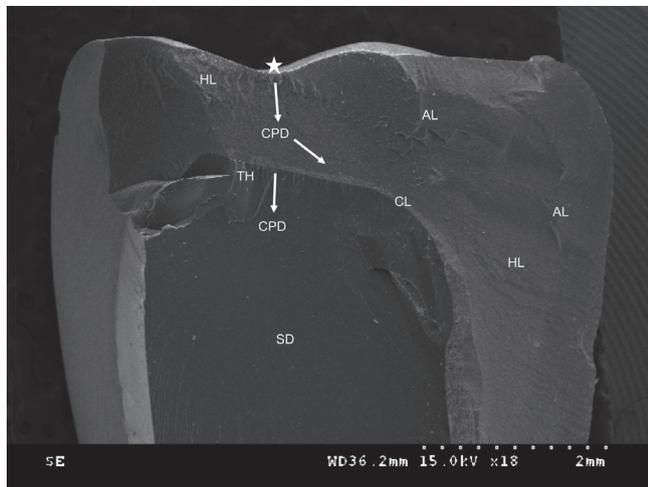
**Fig. 4.** SEM fracture surface image of EN crown with occlusal thickness of 1.0 mm. HL: hackle line, AL: arrest line, white star: origin of fracture, TH: twist hackle, white solid arrow: crack propagation direction (CPD), CL: cementation layer, SD: supporting die.
