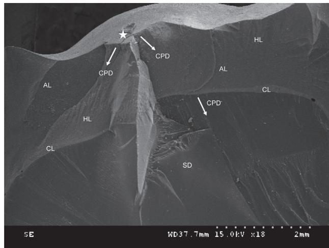
**Fig. 5.** SEM fracture surface image of EN crown with occlusal thickness of 1.5 mm. HL: hackle line, AL: arrest line, white star: origin of fracture, white solid arrow: crack propagation direction (CPD), CL: cementation layer, SD: supporting die.
