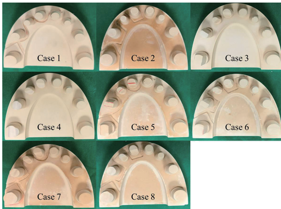
Fig. 3. Dentiform specimen geometry of Cases 1- 8.
