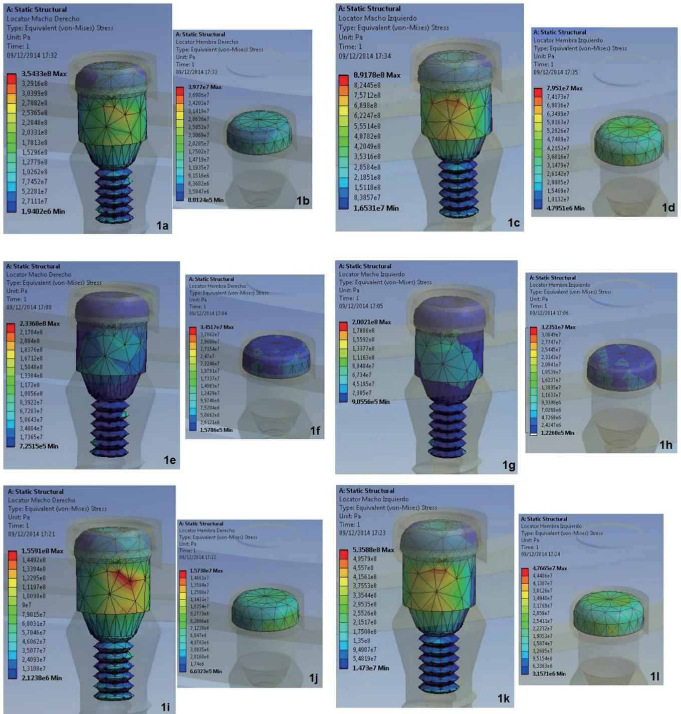
**Fig. 1.** Distribution and location of stress on the abutment and patrx plastic attachment component in the canine level implant model. Above: with unilateral posterior load. Middle: with unilateral midline load. Below: with unilateral canine load. Left half: right side. Right half: left side.
