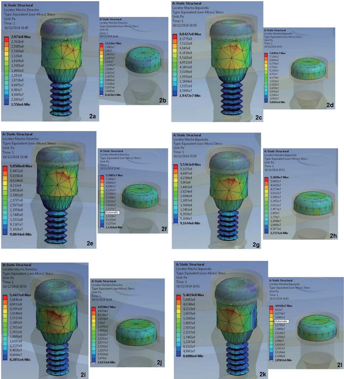
**Fig. 2.** Distribution and location of stress on the abutment and patrix plastic attachment component in the canine level implant model. Above: posterior and midline unilateral combined load. Middle: bilateral posterior load. Below: posterior and midline bilateral combined load. Left half: right side. Right half: left side.
